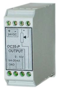
OC35-P has very high accuracy, stability and very attractive price. Potentiometric sensors between  $1k\Omega$  and  $100k\Omega$  can be connected. For rotative sensors the output signal can be calibrated in degrees e.g. 0 ...  $345^{\circ} = 4 - 20mA$ .
